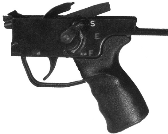
modified HK selective fire trigger housing
